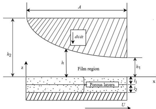
Fig. 1. Double-porous layered slider bearing with parabolic pad surface.
