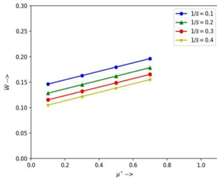
**Fig. 4.** Non-dimensional load carrying capacity against non-dimensional magnetization parameter.
